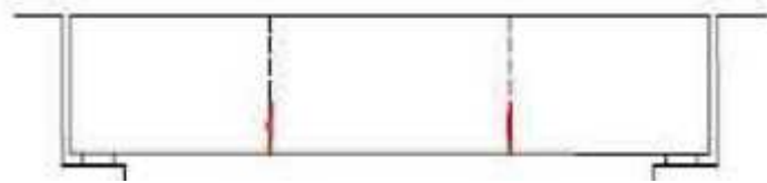
cracks in segment joints
