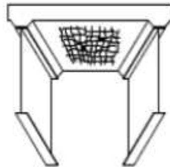
Stage 4 Water penetrates cracks, spalling
