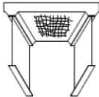
Stage 3 Cracks develop like a mesh
