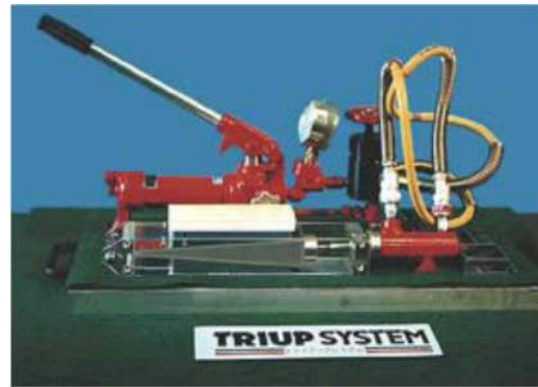
Photo 8-4 50-ton hydraulic jack
