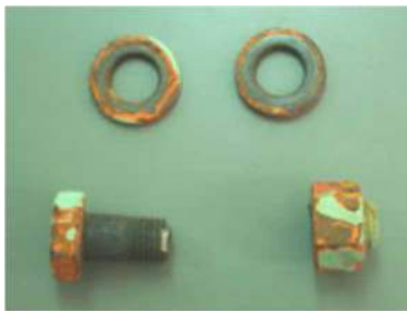
Photo 5-1 Sample bolt with Delayed Fatigue Fracture
