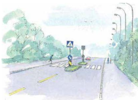
Figure 4-10: Pedestrian crossing with refuge island
