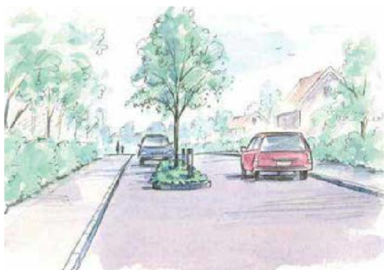
Figure 4-12: Narrowing from two to one lane
