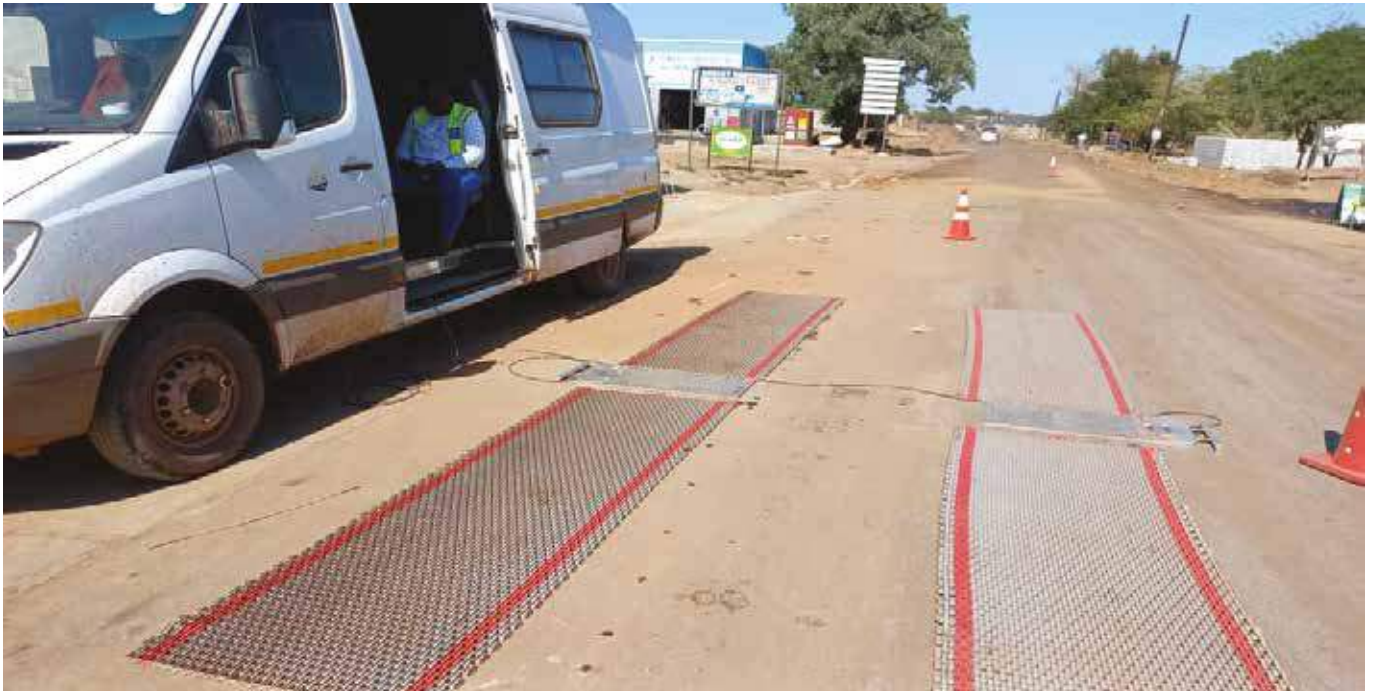
Figure 3.12: A mobile weighbridge mounted to monitor overloads along a township road
