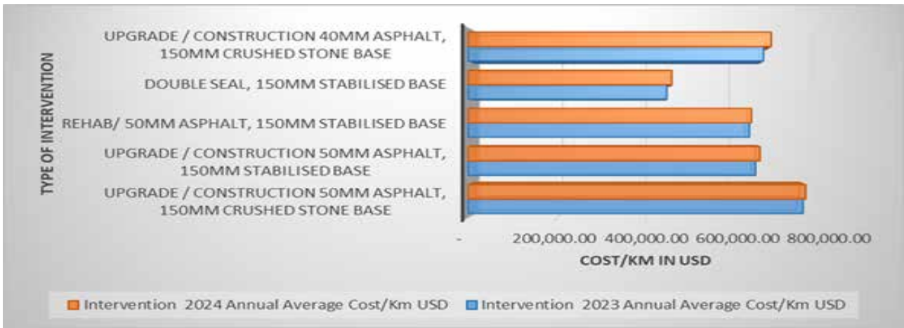
Figure 5.4: Comparative Average Cost Estimates Based on the 1st Principle for 2023 Vis-à-vis 2024 in US$ Per kilometre
