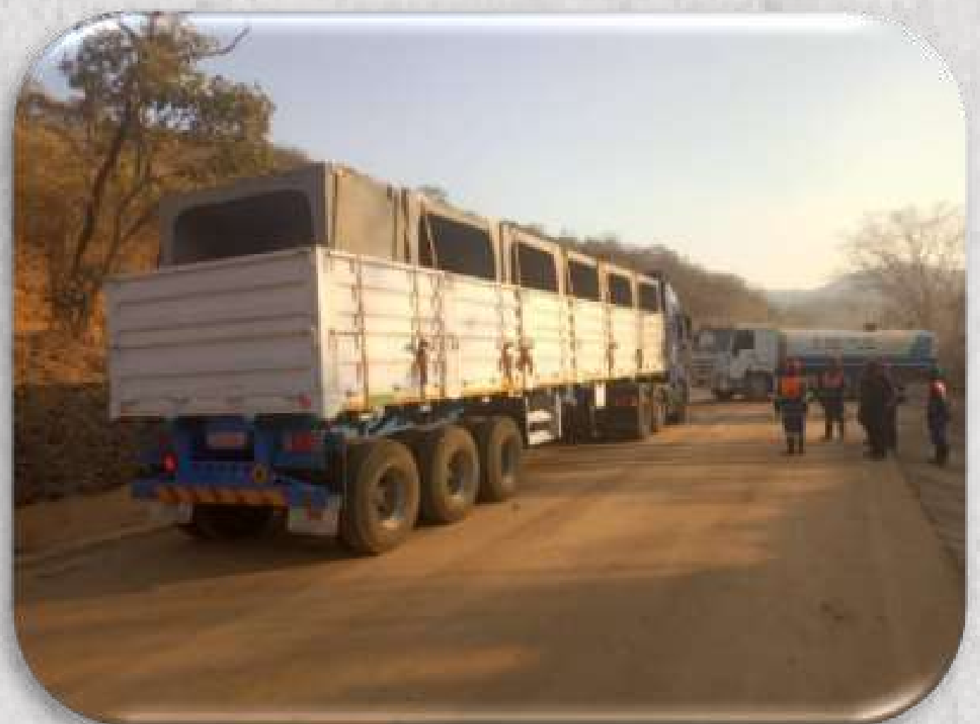
Delivery of 1.8m x 1.8m Box Culverts.
