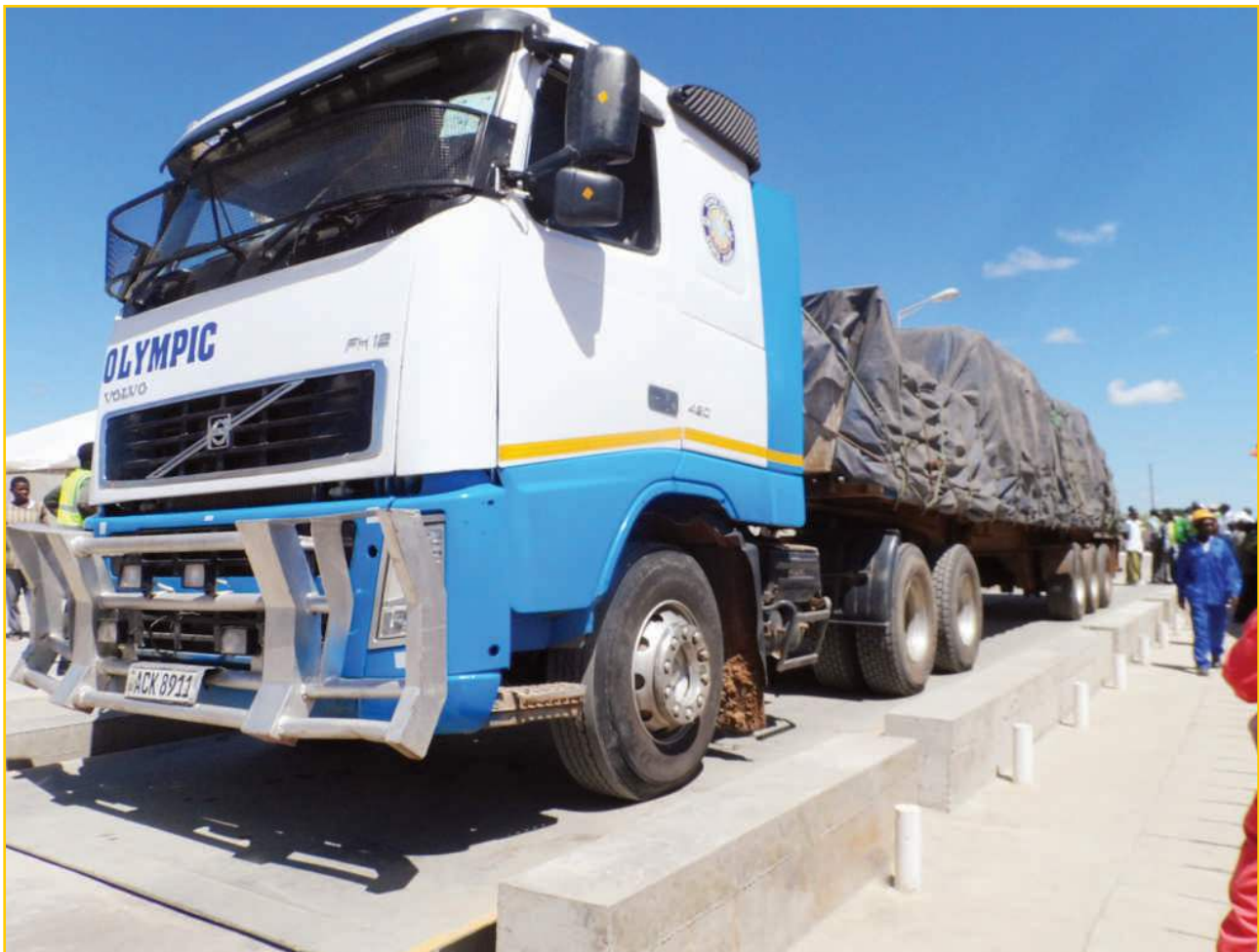
Electronic weighing of the whole truck on a multi-deck to reduce congestion
